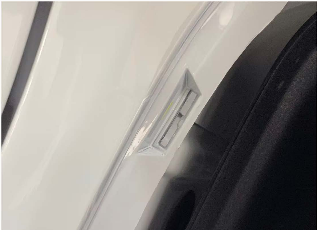
With all the plastic clips depressed while pulling, the Side Scoop should now be free from the rocker panel. (pictured below)
